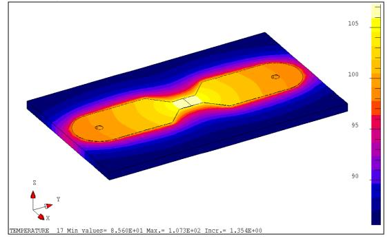
Track thickness 35  $\mu$ m, PCB thickness 1.6 mm,  $T_A$  = 85°C, natural convection,  $I_{PN}$  = 10 A rms or A DC.
